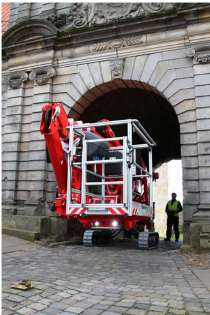
Minimum pass through width of 0,99 m
