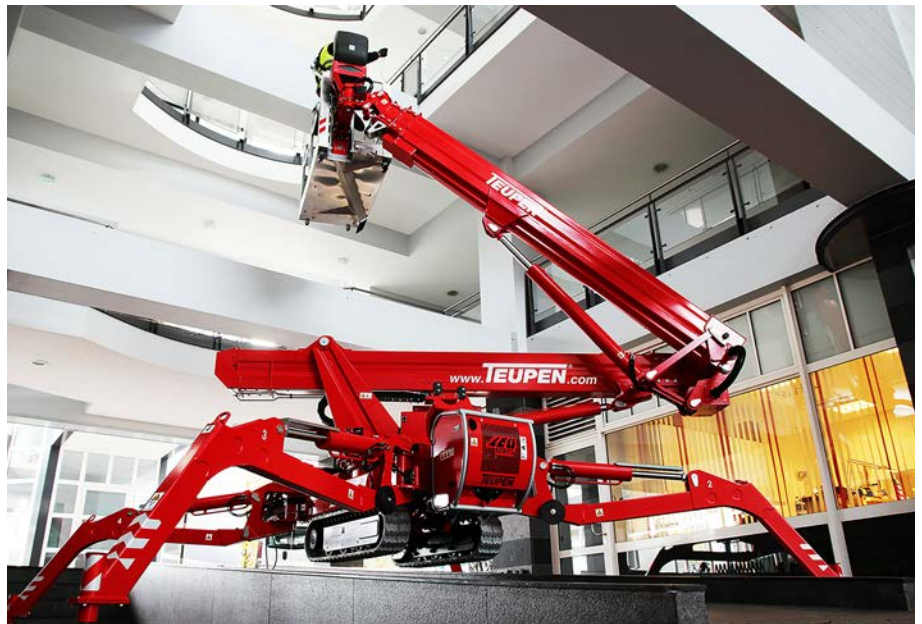
Turntable rotation (450 °) Rotatable platform (2x 90 °)
