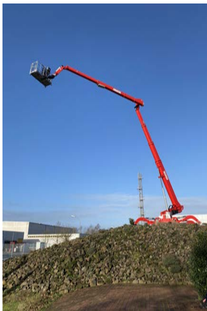
Upper and lower boom can be operated independently
