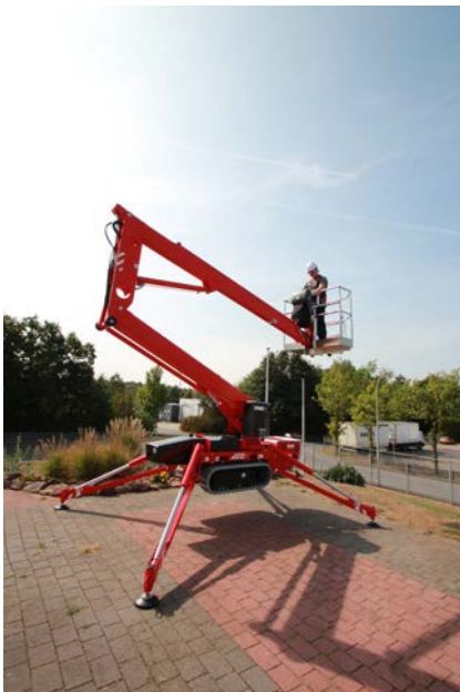
Automatic self-levelling stabiliser system
