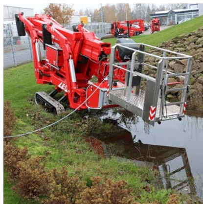
Height- and width adjustable crawler tracks for driving on slopes
