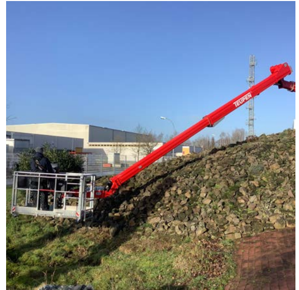
Working in negative areas up to 9,20 m
