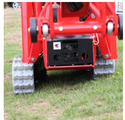
Optional: height- and width adjustable crawler tracks
