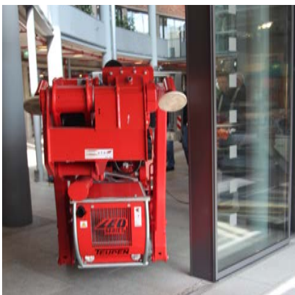
Minimum pass through width of 0,98 m
