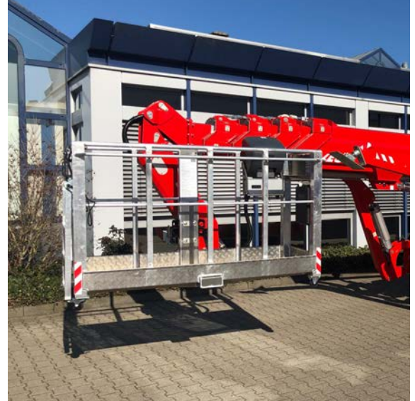
Four different platform sizes available: 900x800 mm, 1200x800 mm, 1500x800 mm, 2000x800 mm
