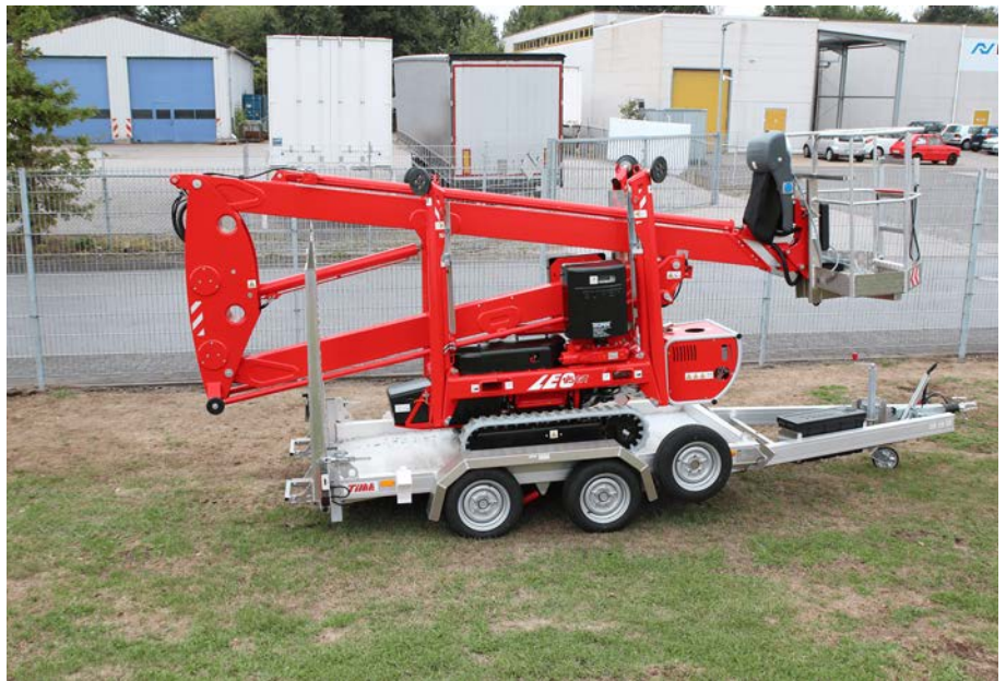
Transportation on a standard trailer possible (2,5-3,0 t)
