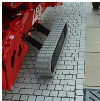
Height- and width adjustable crawler tracks
