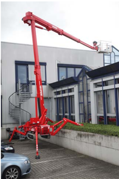
Setting up on ground slopes up to 19,0 ° / 34,0 %
