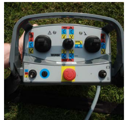
User-friendly cable control with colour coded functions
