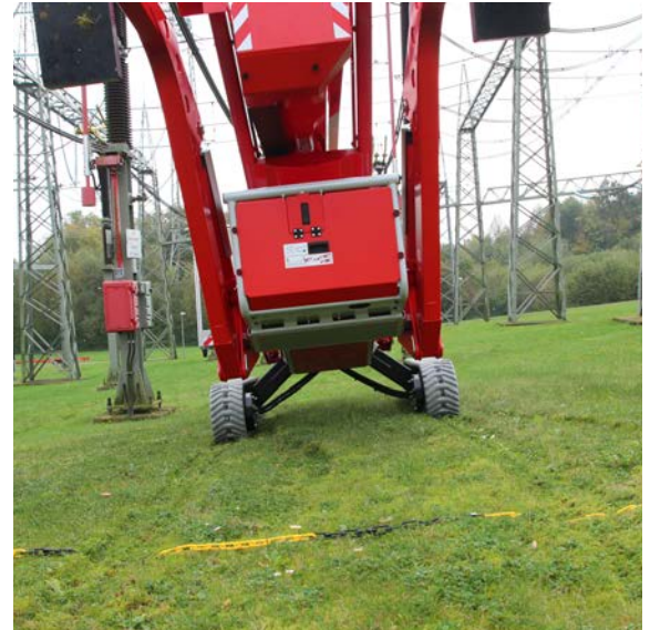
Height- and width adjustable crawler tracks for driving on slopes
