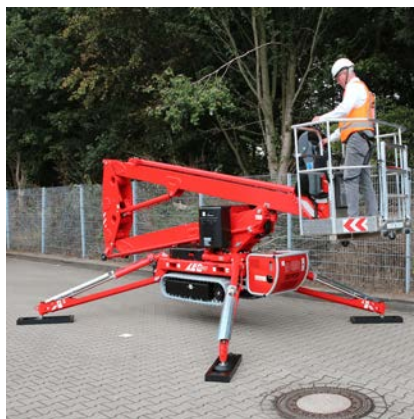
Automatic self-levelling stabiliser system
