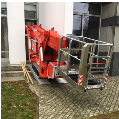
Minimum pass through width of 0,98 m
