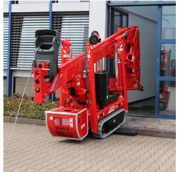
Minimum pass-through width of 0,78 m due to the removable platform
