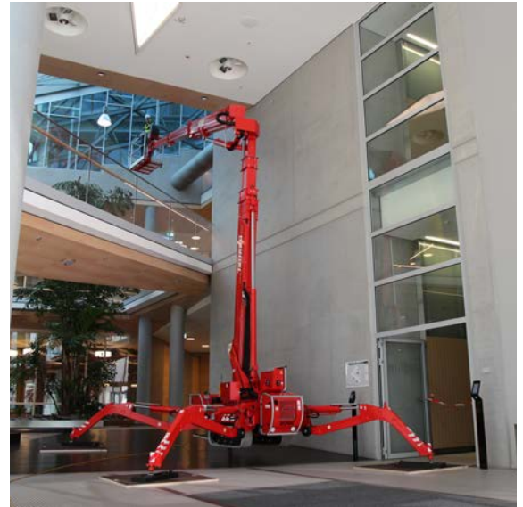
Upper and lower boom can be operated independently for overcoming barriers
