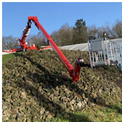
Rotatable platform: 2x 220 ° Movable jib: 200°
