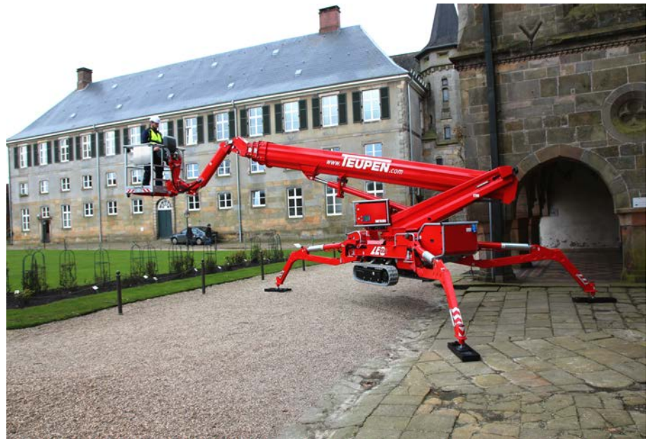
Three different set up positions: Both side wide, both side narrow, one side narrow
