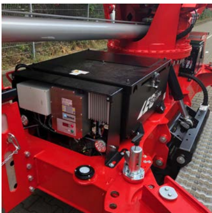
Diesel engine as standard - battery drive optional selectable
