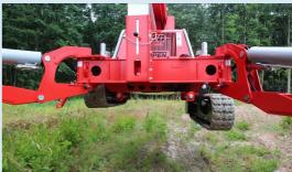
The LEO35Tplus is equipped with height- and width adjustable crawler tracks. It even allows the machine to climb steep slopes and stairs.
