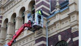
The LE035Tplus features a 180° rotatable platform for more versatility when positioning the platform into tight spots, working alongside façades or in trees.
