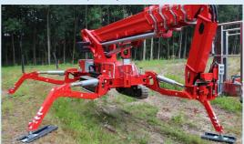
The automatic outrigger system levels out height differences perfectly. Additionally, tree different outrigger setup positions are available.
