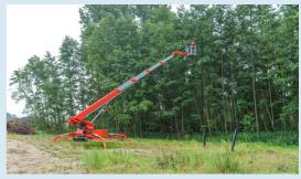
The LE030Tplus features a 180° rotatable platform for more versatility when positioning the platform into tight spots, working alongside façades or in trees.
