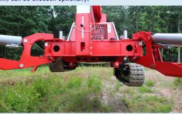
The LEO30Tplus is equipped with height- and width adjustable crawler tracks. It even allows the machine to climb steep slopes and stairs.
