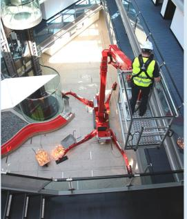
The automatic outrigger system levels out height differences perfectly. Additionally, three different outrigger setup positions are available.
