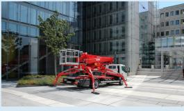
For the transport of the LEO24GT we offer a subframe for a 7,5 t truck. For loading the machine will be lowered about the outrigger system.
