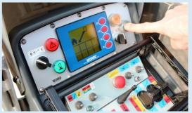
A clearly arranged control panel with interactive display and optional a "Coming home function" for automatic return of boom into transport position.
