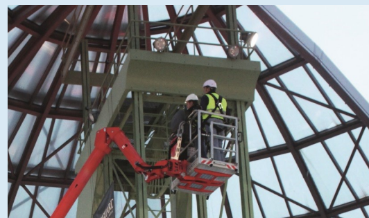
All the new T models features a 180° rotatable platform and a movable jib for more versatility when positioning the platform into tight spots, working alongside façades or in trees.
