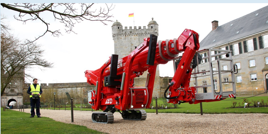
All the new T models features a 180° rotatable platform and a movable jib for more versatility when positioning the platform into tight spots, working alongside façades or in trees.
