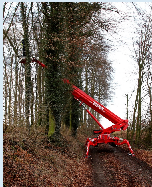
A boom speed control depending on range, swivelling even over narrow outrigger setting. The multi-position stabiliser system offers three different setup positions: Both sides wide, one side wide and one side narrow or both sides narrow.
