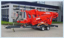
The light LE023GT can be towed on standard trailers. It can either be driven on the trailer or simply use its outrigger system.
