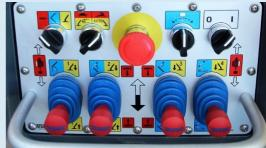
A clearly arranged control panel with color coded functions and only four joysticks for the entire lift operation supports intuitive and safe handling even for inexperienced users.
