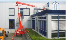
The automatic outrigger system levels out height differences perfectly. Additionally, three different outrigger setup positions are available.
