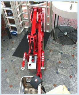
With its compact dimensions the LEO23GT fits through most entrance doors. The sensitive electro-proportional controls allow precise manouevering.
