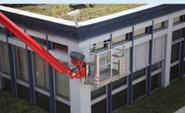
Corner-mounted, 180° turnable platform to swing around obstacles for extra flexibility on the job site.
