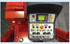
A clearly arranged control panel with interactive display and optional a "coming home function" for automatic return of boom into transport position.
