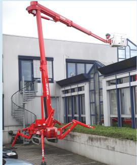
The automatic outrigger system levels out height differences perfectly. Additionally, three different outrigger setup positions are available.
