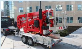
The light LE018GTplus can be towed on standard trailers. With the cable remote control loading is quick and easy.
