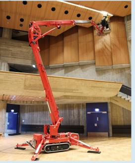
The robust and fully automatic stabiliser system operates with constant ground pressure monitoring directly in the stabiliser plate.
