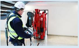
With the cable remote control the operator has a better overview when driving and setting up the lift.
