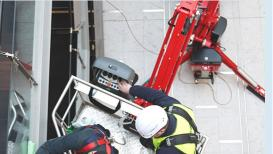
The detachable platform includes a power outlet and an innovative hexagonal shape for easier access to hard-to-reach places.
