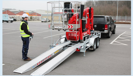
The light LE15GT can be towed on standard trailers. With the cable remote control loading is quick and easy.
