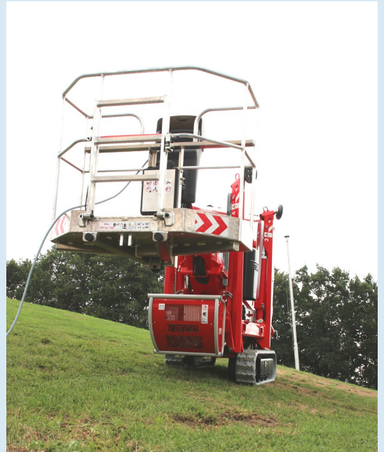
The optional adjustable track chassis allows driving safely alongside slopes and to increase ground clearance for better anibility.
