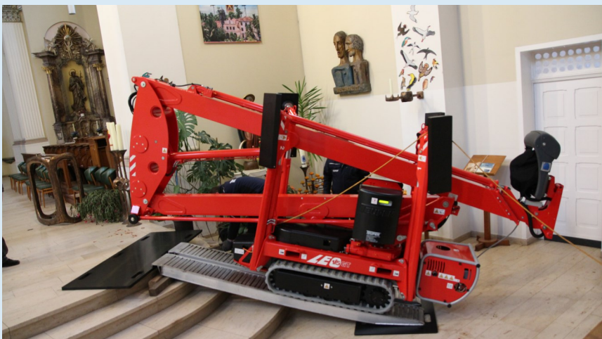
For passing narrow entrances the platform is easily detachable - mounted rollers make moving it around easy.
