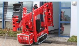
The platform is easily detachable for passing narrow entrances. The cable remote control offers a better overview when operating the crawler tracks.
