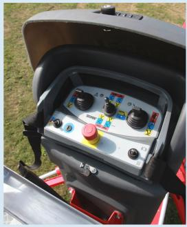
TEUPEN controls are well-arranged with color coded functions. Only two joysticks and one switch for the entire lift operation.
